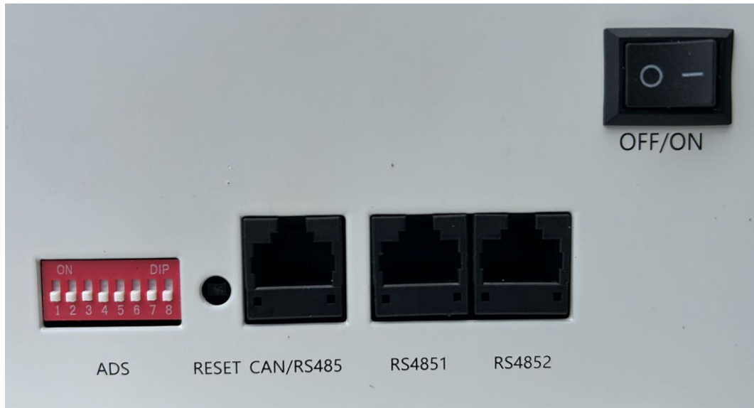
BMS Switch and Connection
